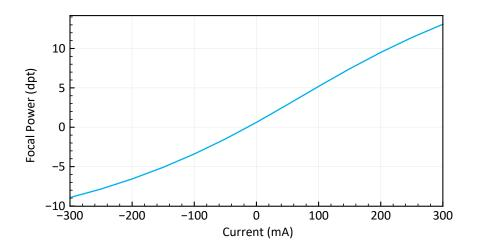
Figure 5: Typical data showing the relation between focal power (in diopters) and electrical current.
