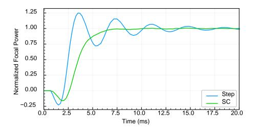
Figure 8: The settling time can be improved with signal conditioning (SC)
