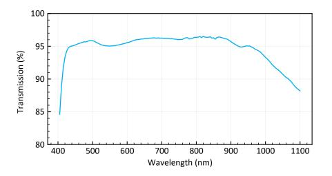
Figure 6: Transmission spectrum of standard EL-12-30-TC.
