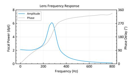
Figure 10 :Typical frequency response and phase delay of the EL-12-30-TC. The driving amplitude is -50 to 50 mA
