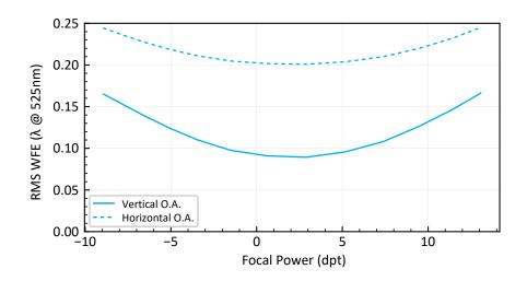
Figure 7: Typical wavefront error of the EL-12-30-TC vs focal power with optical axis vertical and horizontal (@525nm, measured over 80% of the clear aperture).
