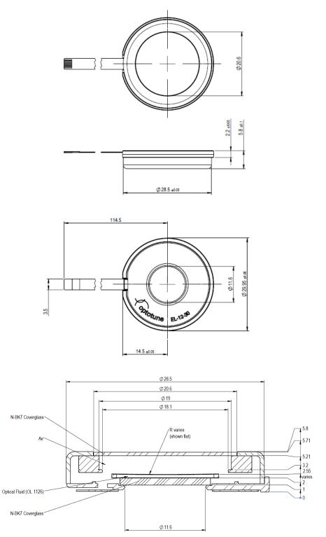
*Figure 1: Mechanical drawing of the EL-12-30-TC*
