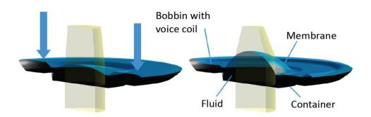
Figure 4: Working principle of the sealed lens container filled with an optical fluid and embedded in an EL-12-30-TC housing.
