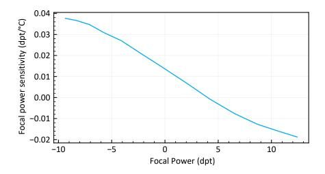
Figure 11: Temperature sensitivity as a function of focal power.
